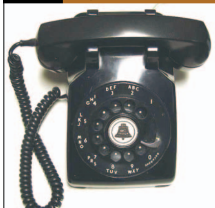
Figure 1 Western Electric 500 C/D rotary dial telephone, circa 1958
